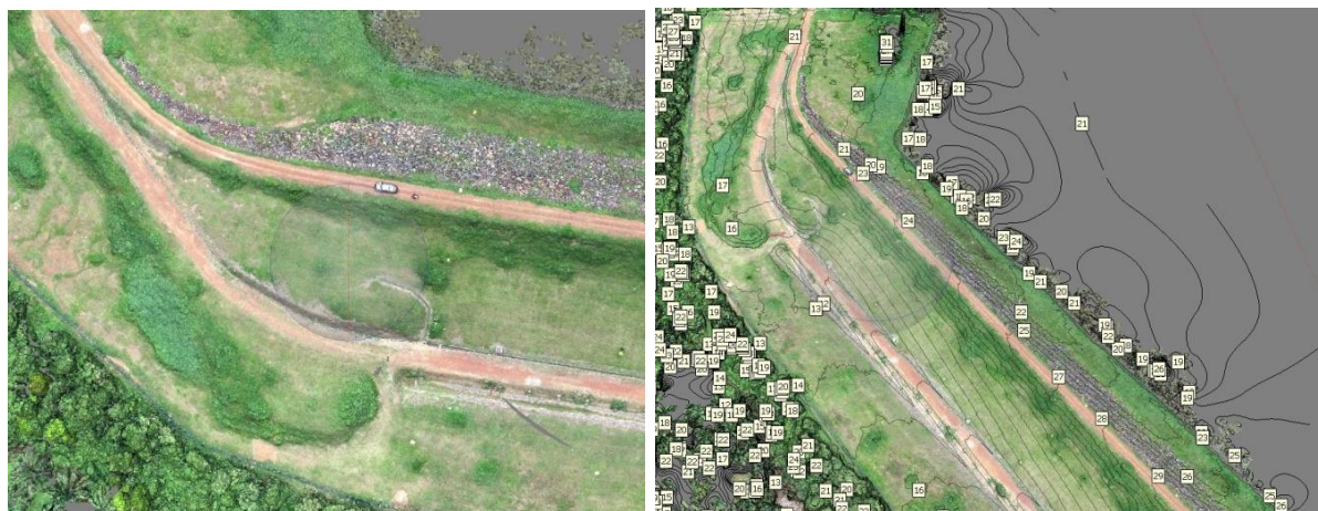
Figure 4.2: Elevation and generation of textured model
