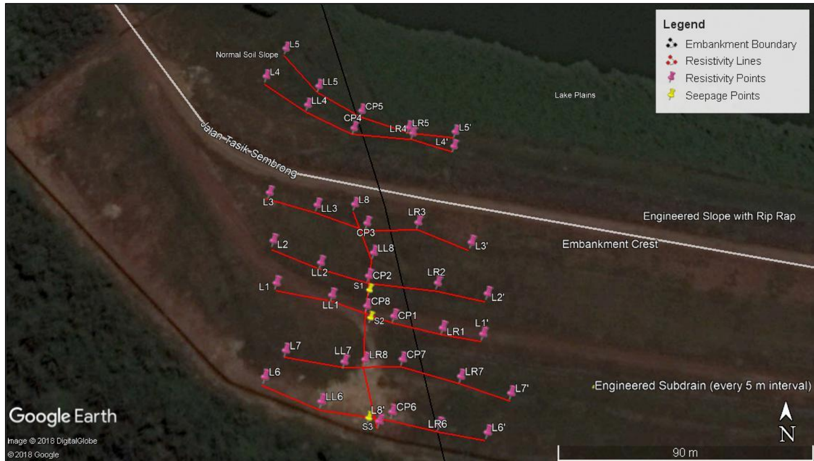
Figure 4.1: Location of electrical resistivity survey lines
